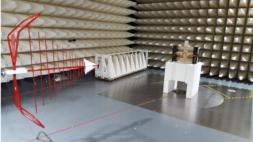
Figure B5. Radiated emission Setup – Low Range 30 to 1000 MHz
