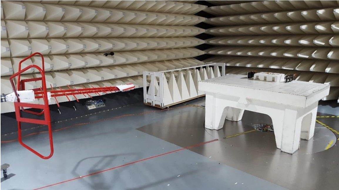
Figure B4: Radiated emission Setup – Low Range 30 to 1000 MHz
