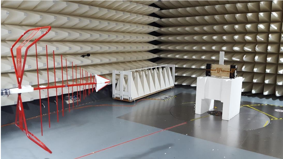
Figure B5. Radiated emission Setup – Low Range 30 to 1000 MHz
