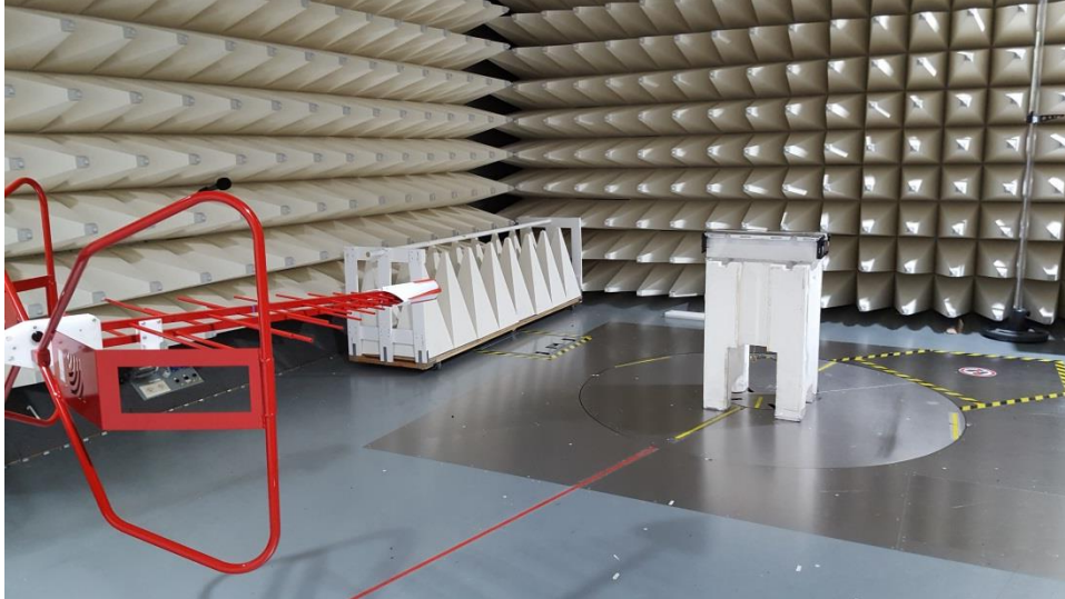
Figure B5. Radiated emission Setup Low range 30MHz to 1GHz (DUT orientation X)
