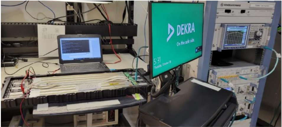
Figure B4. Conducted Test setup
