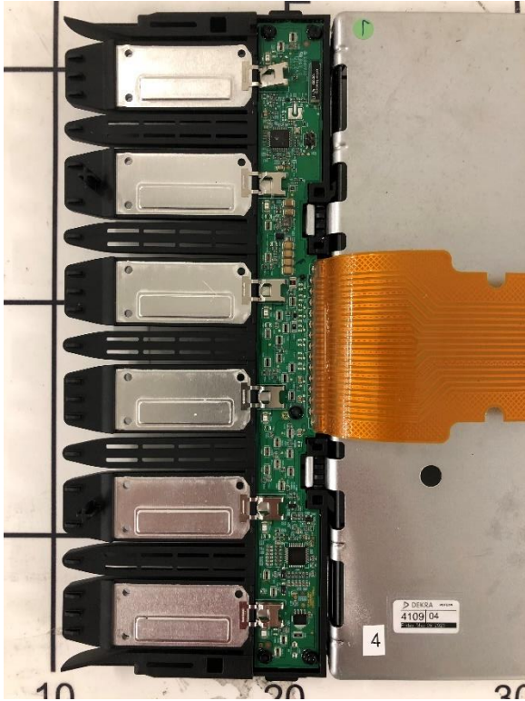
Figure B2. Radiated sample (S/02) – Antenna Port
