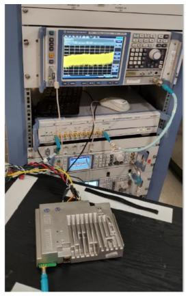
Figure C2. Conducted DUT Test setup
