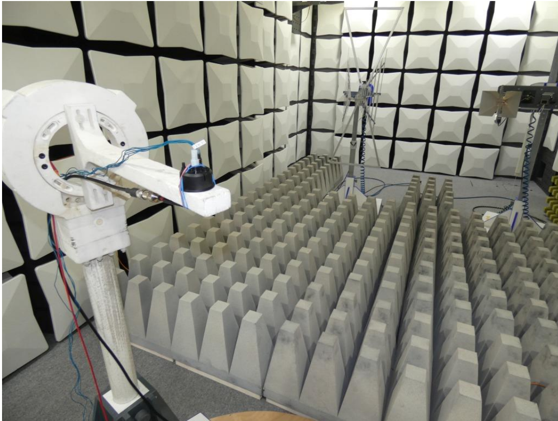
Photo 3: Test setup for radiated measurements (1 GHz – 26 GHz)
