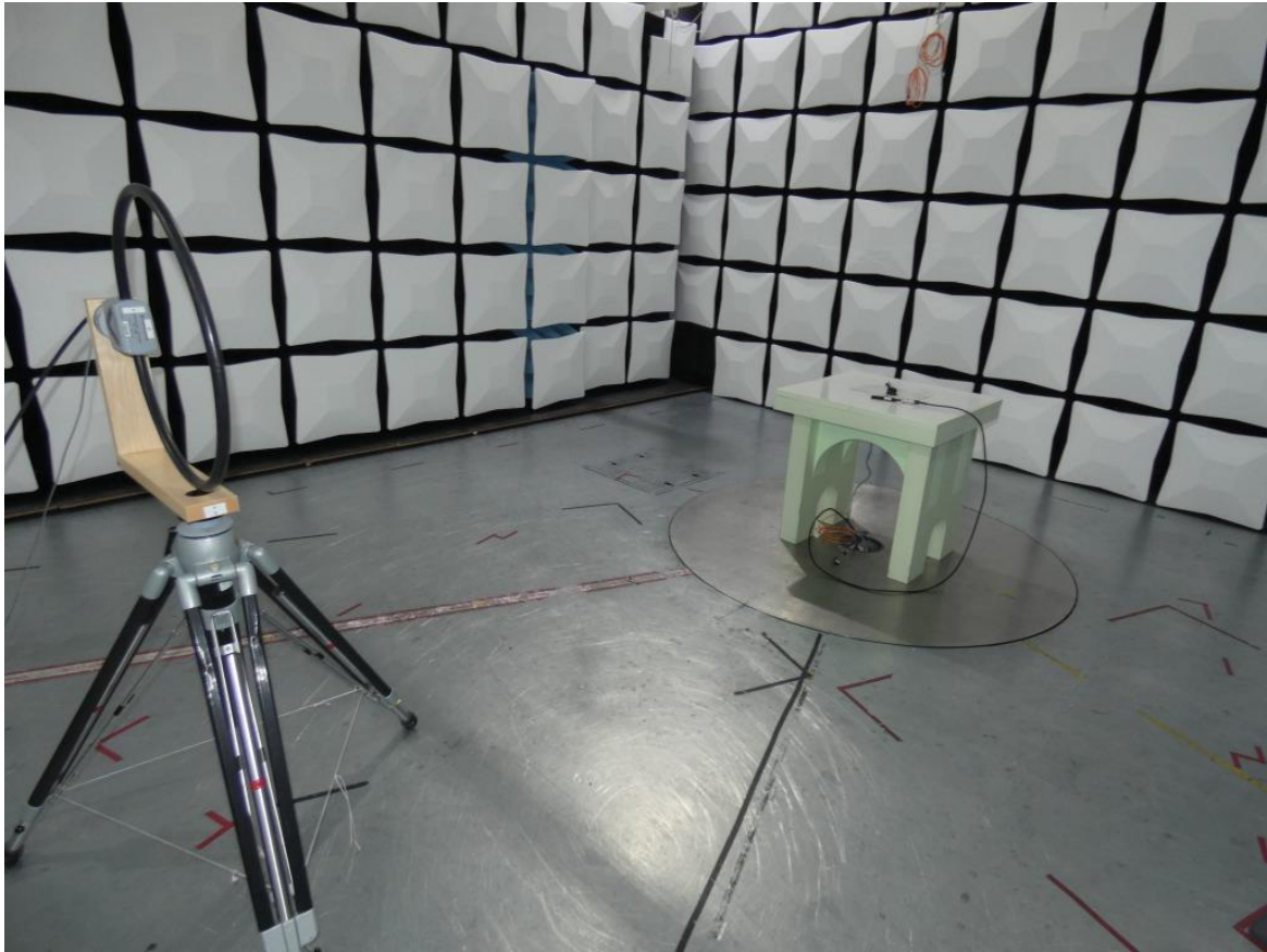
Photo 1: Test setup for radiated measurements (9 kHz - 30 MHz)
