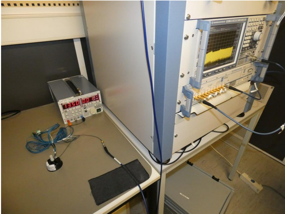
Photo 5: Test setup for conducted measurements on R&S TS8997
