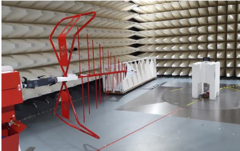
Figure B5. Radiated emission Setup 1
