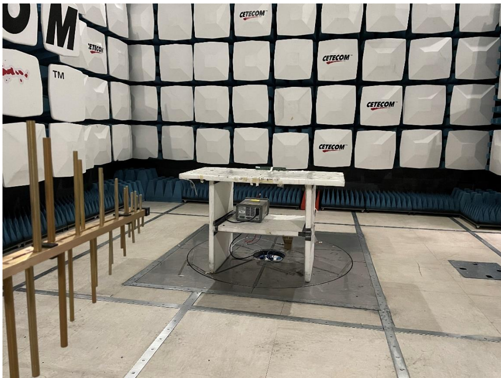
Photo 2: Emissions in frequency range 30 MHz to 1 GHz
