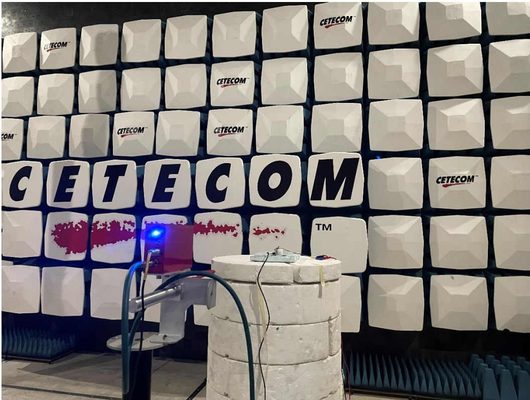
Photo 5: Emissions in frequency range 18-40 GHz
