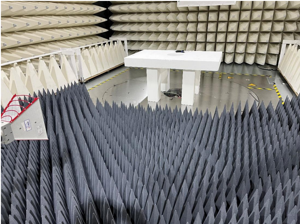
9. Radiated Emission test setup High Range
