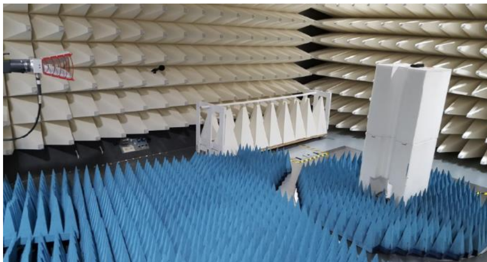
Figure B2. EIRP Radiated Test Setup
