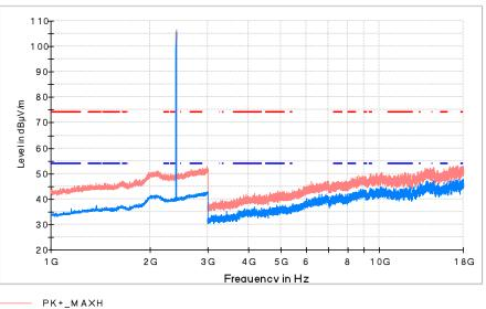
TX limits to Spurious Emission FCC15.247(1-26G) Restricted Bands AVG Limit TX limits to Spurious Emission FCC15.247 Restricted Bands PK Limit RMS\_MAXH
