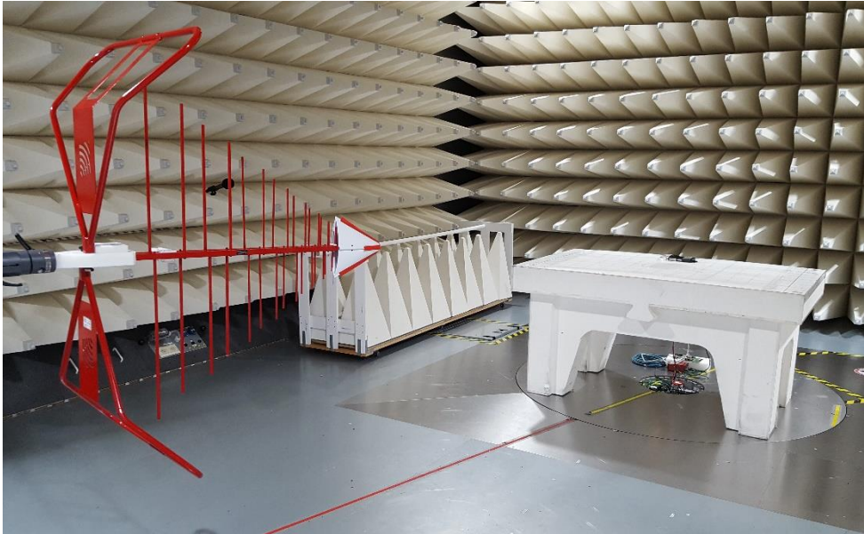
Figure B5. Radiated emission Setup 1 – Low Range 30 to 1000 MHz
