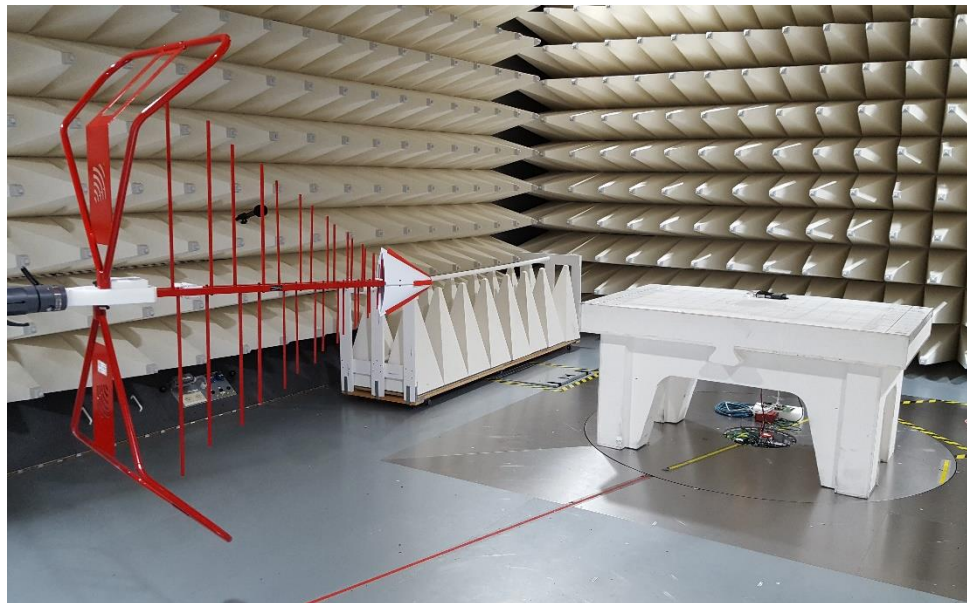
Figure B5. Radiated emission Setup 1 – Low Range 30 to 1000 MHz
