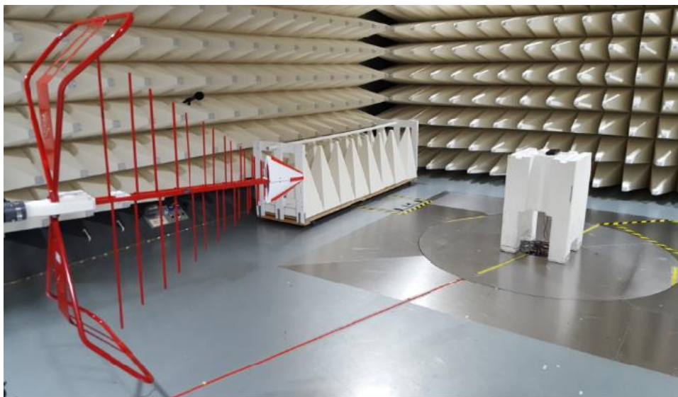
Figure B6. Radiated emission Test Setup 1
