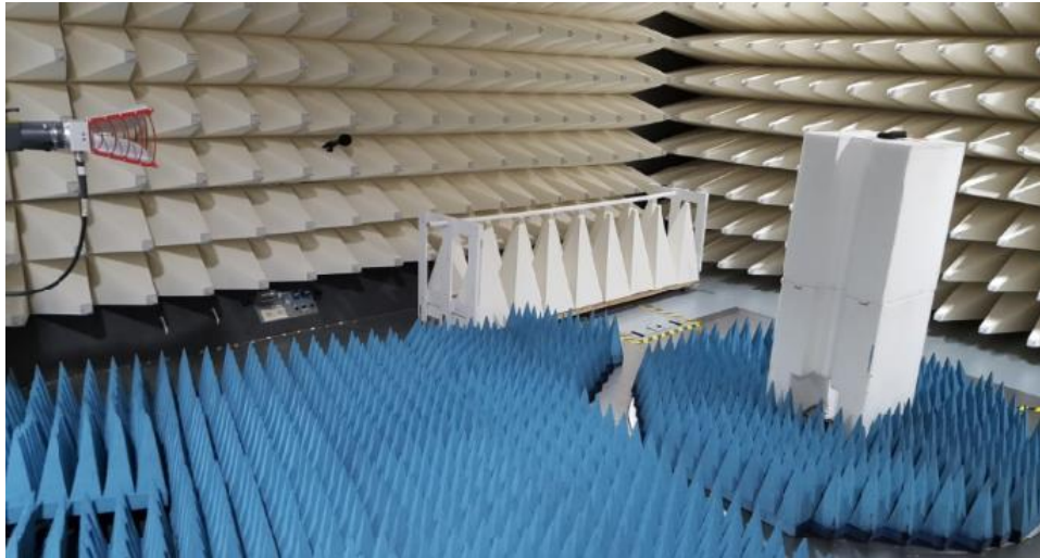
Figure B7. Radiated emission Test Setup 2
