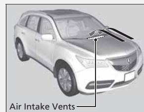
Air Intake Vents
