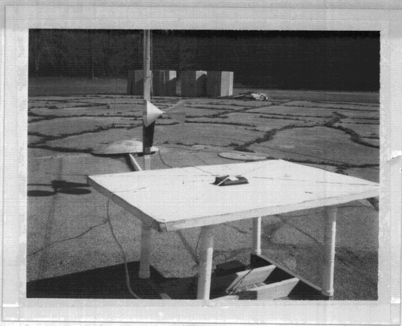
Figure 5.4. DUT on the open-site test table showing the worst case position and orientation with respect to the measuring antenna at "fundamental".
