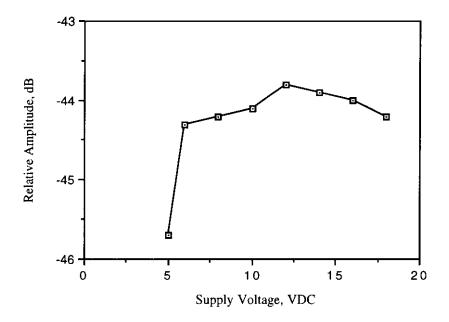
Figure 6.2. Relative emission at "fundamental" vs. supply voltage.
