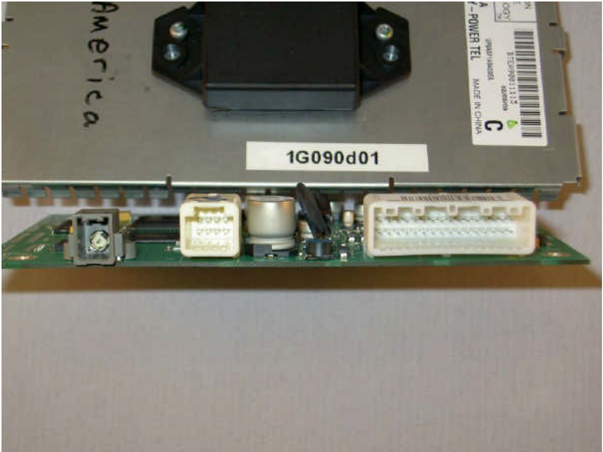
Photo 8: Interfaces of EUT (lefthand side: antenna connector) The photo does not show one of the tested samples.
