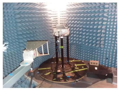
Figure 3: Radiated Emissions, 1GHz – 18GHz Test Setup Photo
