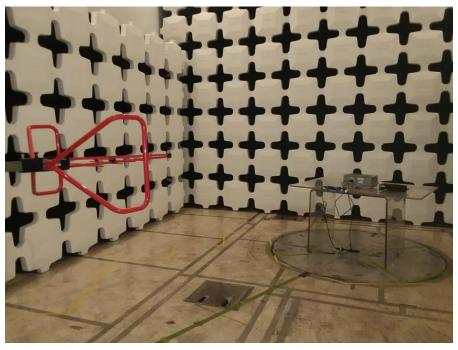
Figure 2: Radiated Emissions, 30MHz – 1GHz Test Setup Photo
