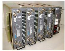
The 125W Dual Amplifier Booster and Dual Amplifier Combiner Modules are integral components of Communication Component Inc.'s Cellular GSM-EDGE Cell Booster System. The Cell Booster System provides the means to add capacity or increase the coverage area and penetration of existing GSM-EDGE sites. The 125W Dual Amplifier Combiner (DAC) module combines multiple GSM channels onto a common antenna port with-
