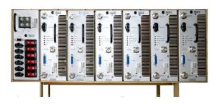
The 125W Dual Amplifier Booster and Dual Amplifier Combiner Modules are integral components of Communication Component Inc.'s PCS GSM-EDGE Cell Booster System. The Cell Booster System provides the means to add capacity or increase the coverage area and
