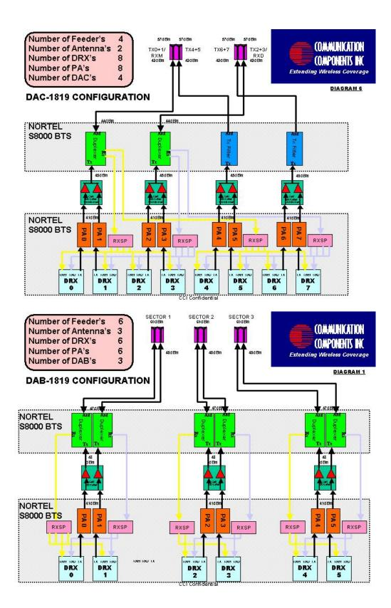
Although the gain of the Dual Amplifier Booster/ Combiner is fixed, the output can be adjusted by setting the input power level. The input to the Dual Amplifier Booster/ Combiner is the Nortel Power Amplifier (PA) whose output can be set at 16 power levels in 2dB increments. As shown in diagram #1 and #2, setting the output level of the PA to 41 dBm will result in a power level at the output of the Dual Amplifier Booster/ Combiner of 45.5 dBm in the combined mode.
