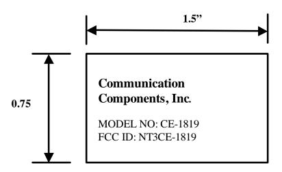
This drawing represents the label that will be affixed to the side or to the front of the Cell Extender case. This label will be printed on a mylar material which has been selected to last the life of the product.
