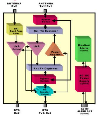
The CE-1819 PCS Band Extender connects directly to a Base Station Transmitter. The Forward Transmit Path is the only path that transmits wirelessly. Antenna RX2 on the diagram above is for an Uplink path to the BTS. The BTS TX out does not connect to the BTS RX2 port.
