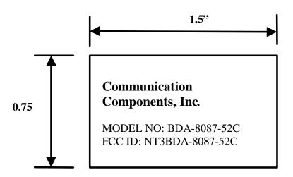
This drawing represents the label that will be affixed to the front of the amplifier case. This label will be printed on a mylar material which has been selected to last the life of the product.
