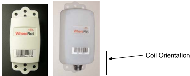
Figure 5 The WhereTag III and WhereTag III ST The solid line shows the orientation of the pick up coil for both WhereTags.
