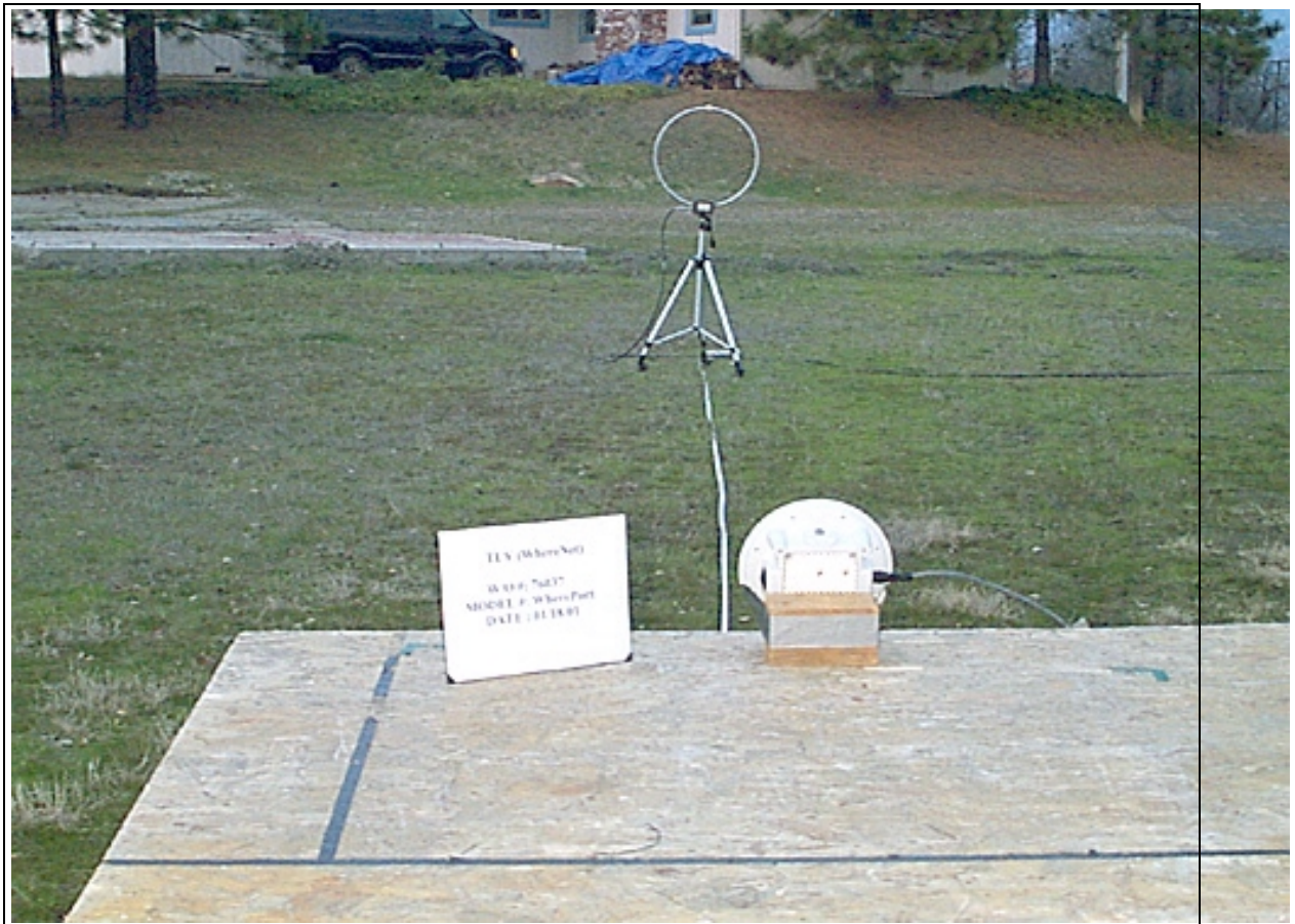
Radiated Emissions - Back View (Mag Loop Antenna)
