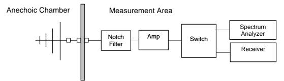
The product was initially tested to find worst case orientation for the maximization of spurious emissions. Worst case orientation was used for all emission testing.
