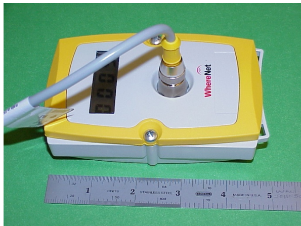
Figure 1 Photograph of the WhereCall III+ PLC with an interface cable attached. (This cable is not included with the WhereCall III+ PLC.)
