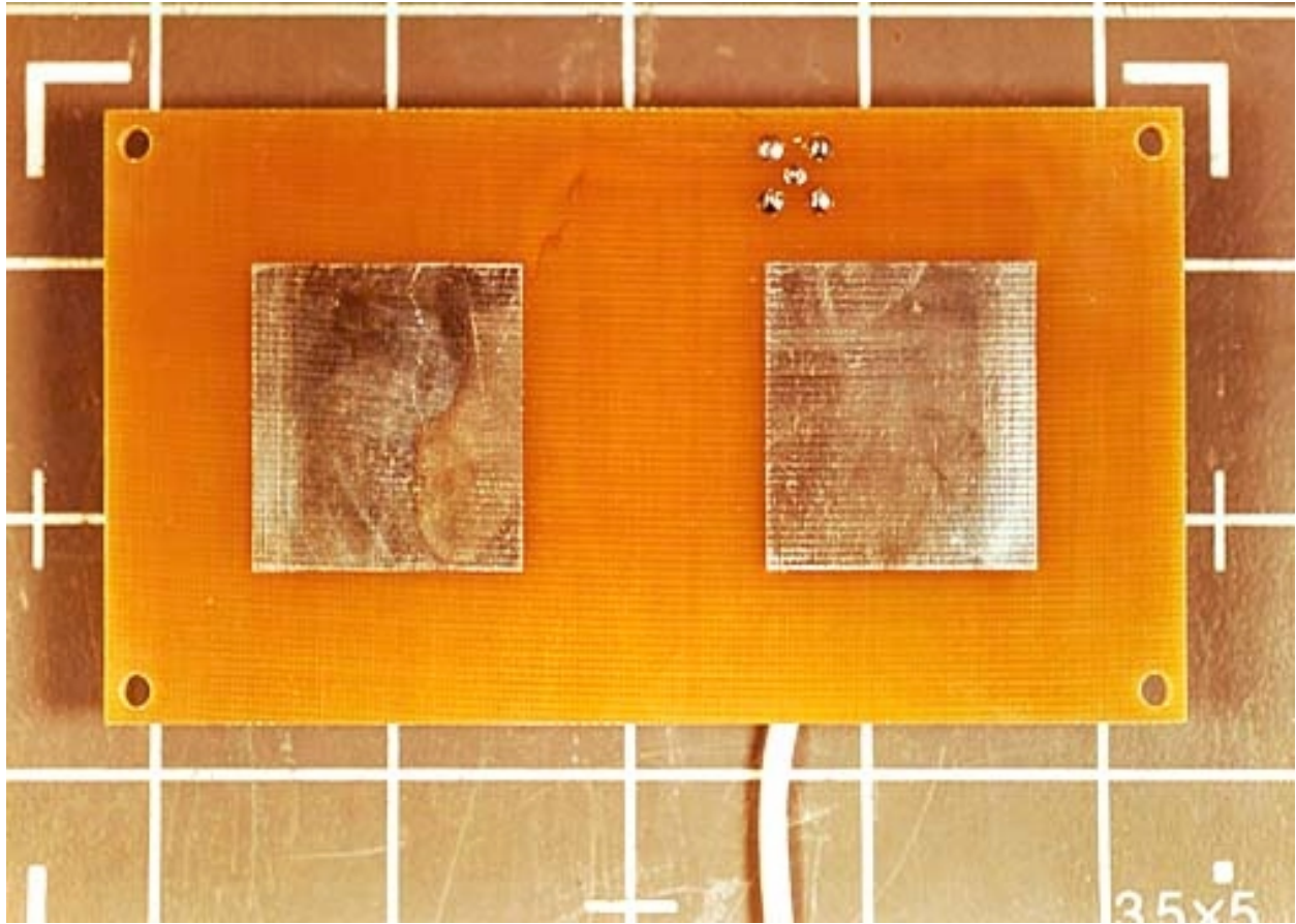
Top PCB in Patch Antenna
