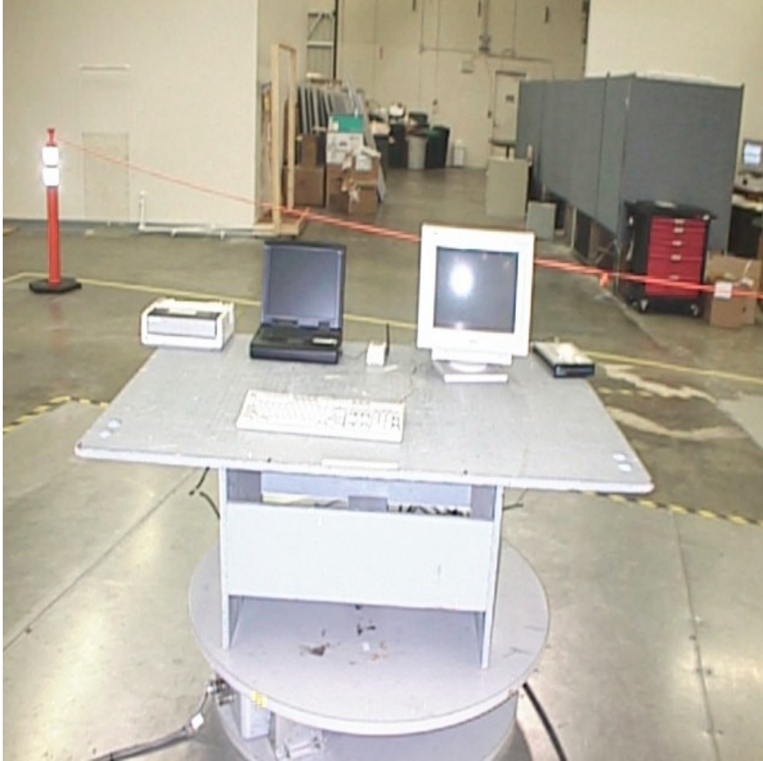
RADIATED EMISSIONS TEST SETUP; FRONT SIDE
