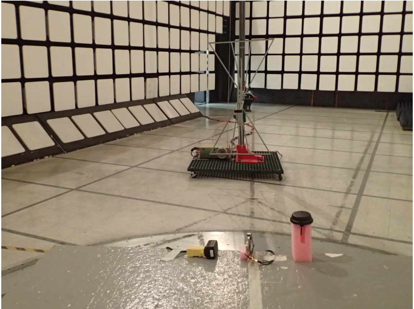
Radiated Emissions @ 3 m EUT with 4 dBi Puck Antenna, Orthogonal Position 1
