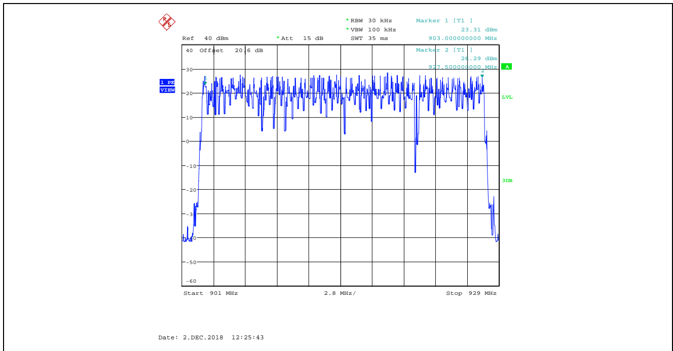
Plot 5.3.4.24. Number of Hopping Frequencies, High Data Rate, 500 kHz CS The Total Number of Hopping Channel in 902 – 928 MHz Band is 50 (14 + 20 + 16)
