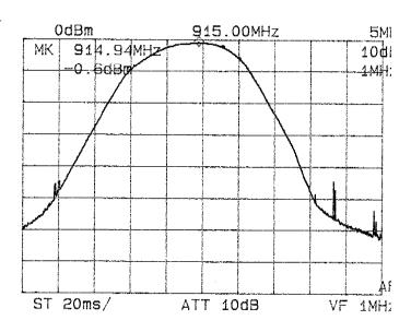
PEAK POWER OUTPUT AT ANTENNA TERMINAL - SET CHANNEL 64
