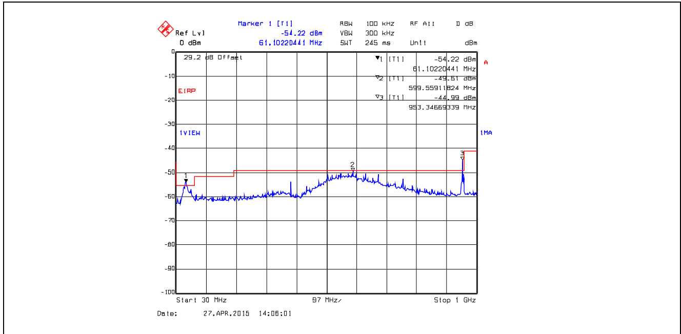
Plot 5.4.4.13. Conducted Spurious Emissions in Restricted Frequency Bands 802.11b, Ch 11, 2462 MHz, CCK 11 Mbps, TX Gain Setting 35, Peak Detector Markers 1, 2 & 3 are outside of RB
