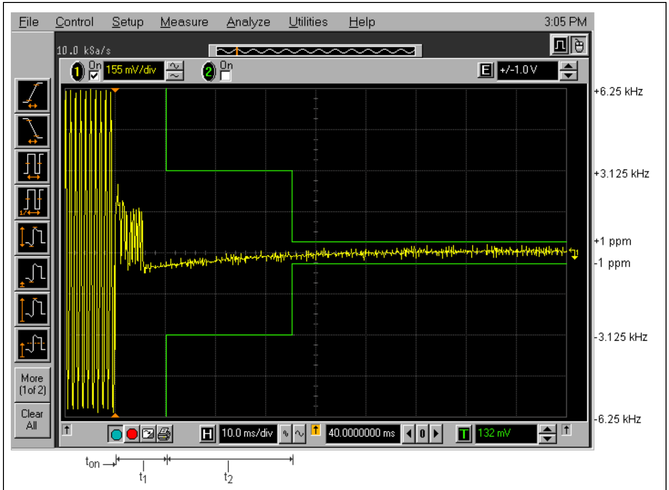
Plot 5.7.4.3. Transient Frequency Behavior on 6.25 kHz Channel Spacing Test Frequency: 410.05 MHz; Power: 2 W; Test Conditions: Switch on condition t_{on} , t_1 , and t_2
