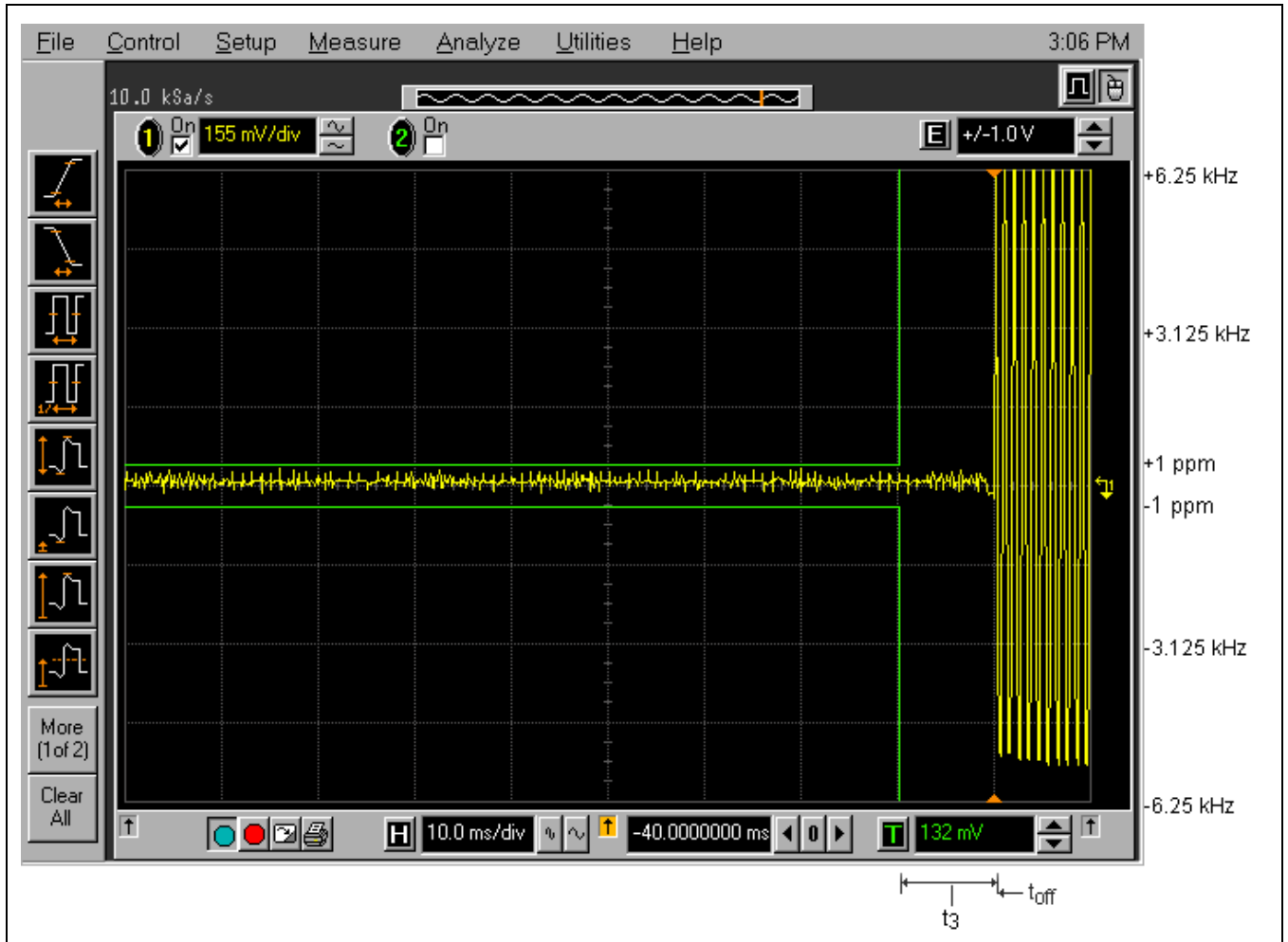
Plot 5.7.4.4. Transient Frequency Behavior on 6.25 kHz Channel Spacing Test Frequency: 410.05 MHz; Power: 2 W; Test Conditions: Switch off condition t_3 , t_{off}
