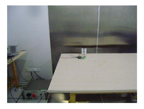
Radiation Emission Test Setup (30MHz to 1GHz)
