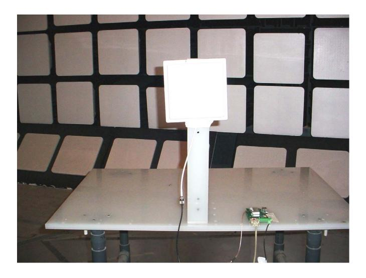
Radiated Emissions @ 3 Meters EUT with 14 dBi Patch Antenna
