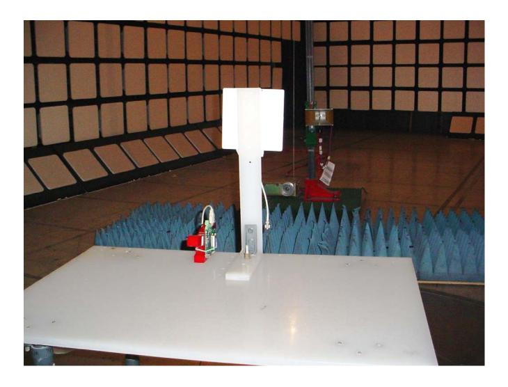
Radiated Emissions @ 3 Meters EUT with 14.5 dBi Yagi Antenna
