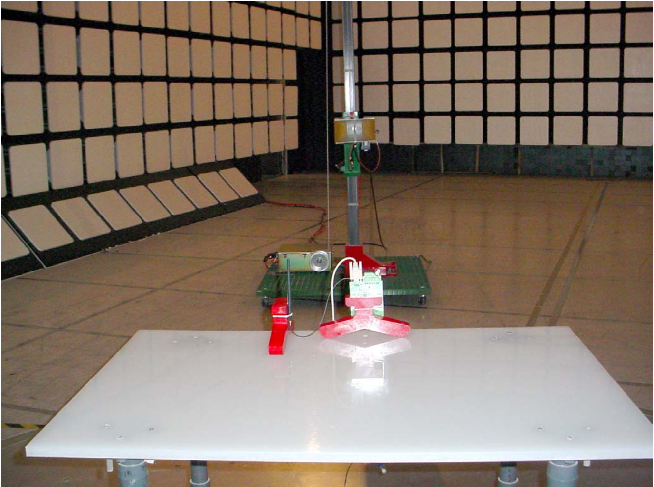
Radiated Emissions @ 3 m EUT with Quarter Wave Antenna, 1.5 dBi Gain
