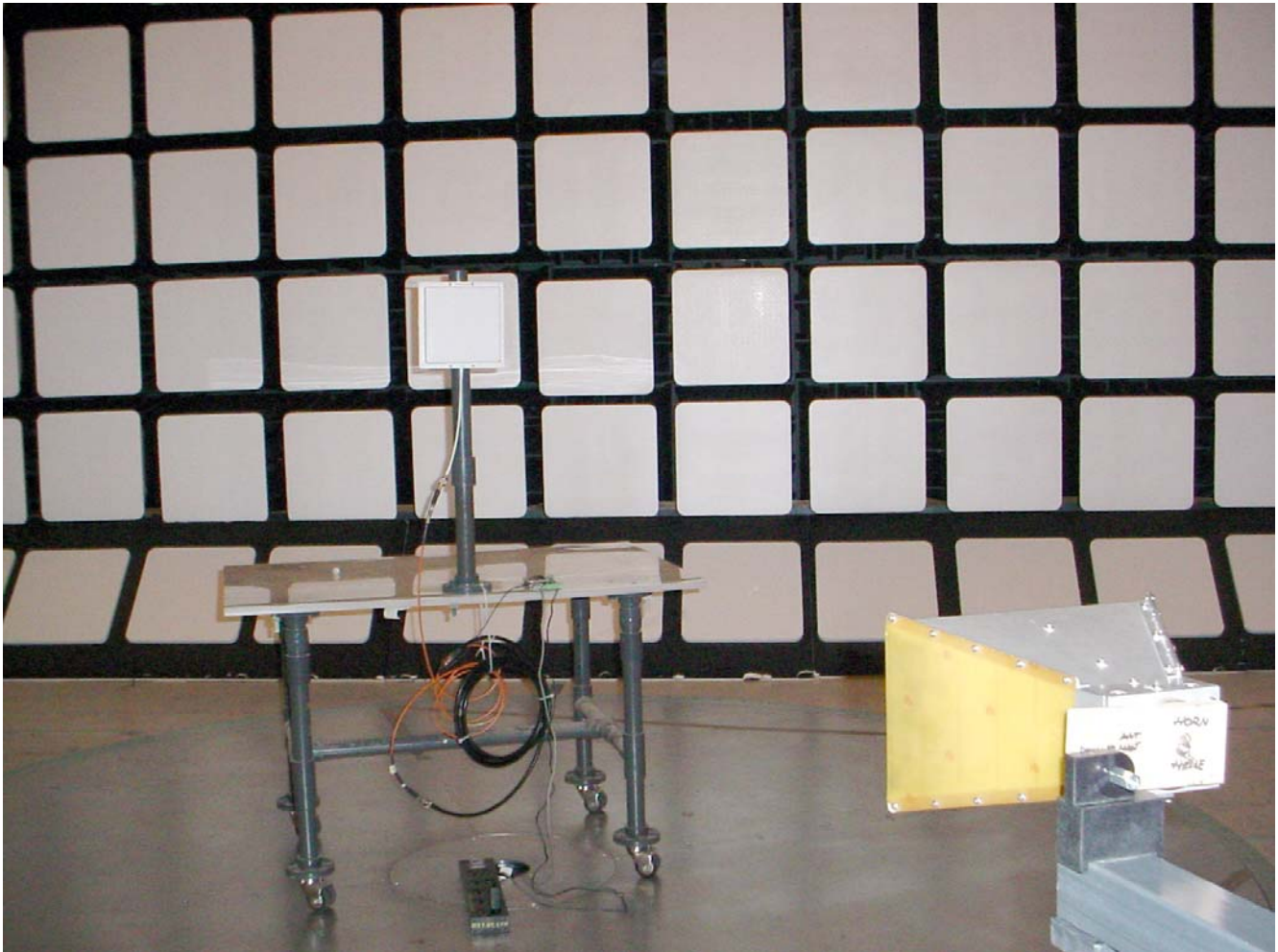
Radiated Emissions @ 3 Meters EUT with 14 dBi Patch Antenna
