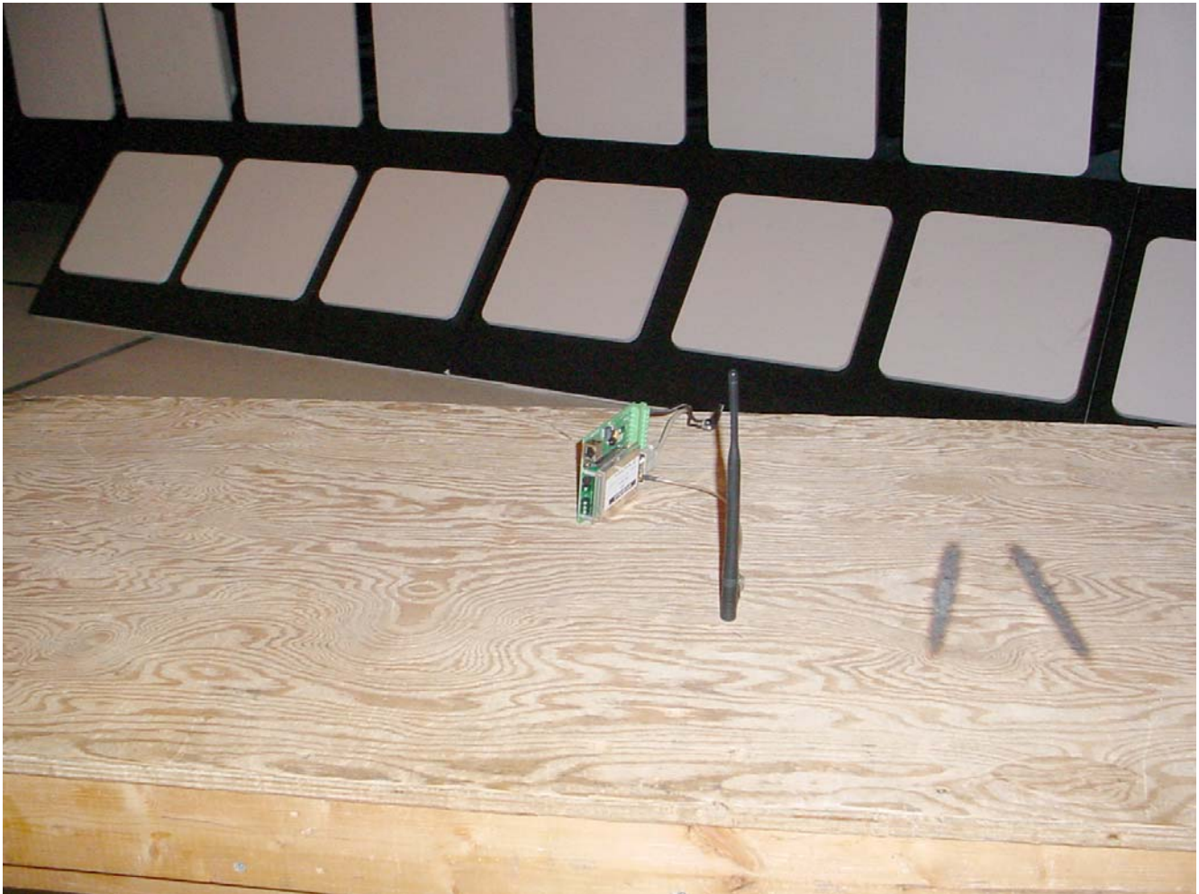
Radiated Emissions @ 3 Meters EUT with Rubber Ducky Antenna, 2 dBi Gain
