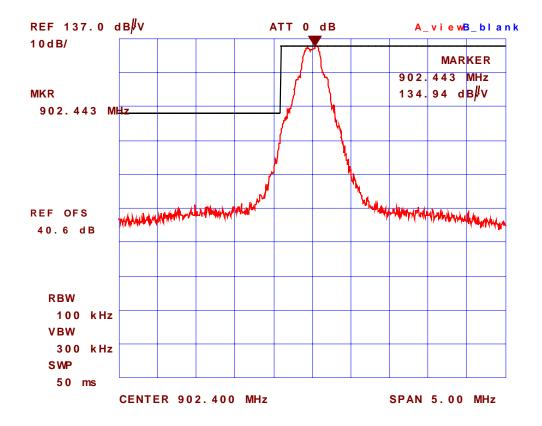
Plot #51: Band-Edge Radiated Emissions @ 3 meters, Rx Antenna: Horizontal Test Configuration # 4: Microhard MHX920 with Omni Directional Antenna, Microhard P/N: MHS031471, Gain: 6 dBd, Highest channel frequency: 927.6 MHz
