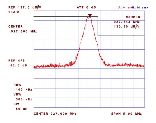
Plot #52: Band-Edge Radiated Emissions @ 3 meters, Rx Antenna: Vertical Test Configuration # 4: Microhard MHX920 with Omni Directional Antenna, Microhard P/N: MHS031471, Gain: 6 dBd, Highest channel frequency: 927.6 MHz
