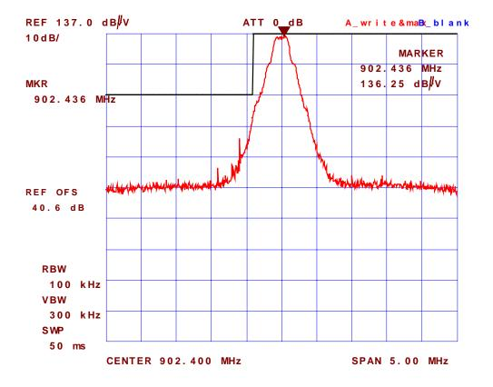
Plot #55: Band-Edge Radiated Emissions @ 3 meters, Rx Antenna: Horizontal Test Configuration # 5: Microhard MHX920 with Yagi Antenna, Microhard P/N: MHS031441, Gain: 12 dBd, Highest channel frequency: 927.6 MHz
