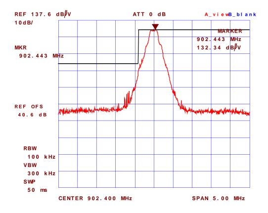
Plot #43: Band-Edge Radiated Emissions @ 3 meters, Rx Antenna: Horizontal Test Configuration # 2: Microhard MHX920 with Rubber Ducky Swivel Antenna, Microhard P/N: MHS031000, Gain: 2 dBi, Highest channel frequency: 927.6 MHz
