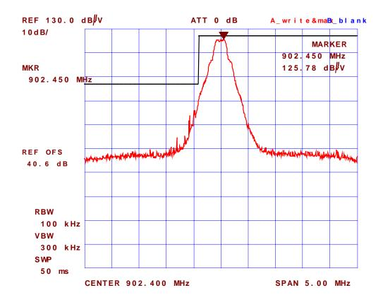
Plot #47: Band-Edge Radiated Emissions @ 3 meters, Rx Antenna: Horizontal Test Configuration # 3: Microhard MHX920 with Transit Antenna, Microhard P/N: MHS031220, Gain: 3 dBd, Highest channel frequency: 927.6 MHz
