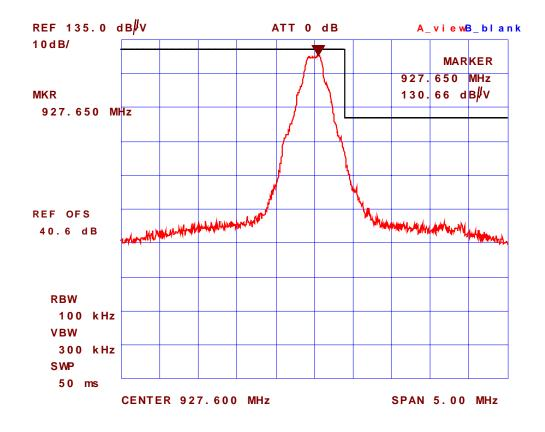
Plot #45: Band-Edge Radiated Emissions @ 3 meters, Rx Antenna: Horizontal Test Configuration # 3: Microhard MHX920 with Transit Antenna, Microhard P/N: MHS031220, Gain: 3 dBd, Lowest channel frequency: 902.4 MHz
