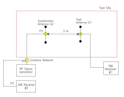
P3 = P2 + Insertion Loss (P1-P3EIRP = P3 + G2 Use the following spectrum analyzer settings:
