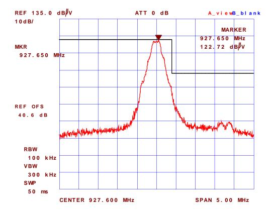
Plot #44: Band-Edge Radiated Emissions @ 3 meters, Rx Antenna: Vertical Test Configuration # 2: Microhard MHX920 with Rubber Ducky Swivel Antenna, Microhard P/N: MHS031000, Gain: 2 dBi, Highest channel frequency: 927.6 MHz
