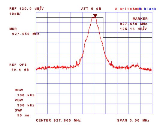
Plot #48: Band-Edge Radiated Emissions @ 3 meters, Rx Antenna: Vertical Test Configuration # 3: Microhard MHX920 with Transit Antenna, Microhard P/N: MHS031220, Gain: 3 dBd, Highest channel frequency: 927.6 MHz
