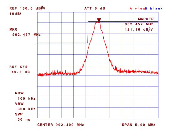
Plot #38: Band-Edge Radiated Emissions @ 3 meters, Rx Antenna: Vertical Test Configuration # 1: Microhard MHX920 with ¼ Wave Antenna, Microhard P/N: MHS031060, Gain: 1.5 dBi Microhard, Lowest channel frequency: 902.4 MHz
