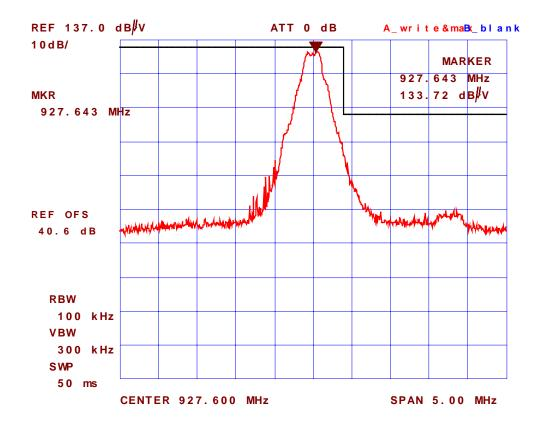
Plot #53: Band-Edge Radiated Emissions @ 3 meters, Rx Antenna: Horizontal Test Configuration # 5: Microhard MHX920 with Yagi Antenna, Microhard P/N: MHS031441, Gain: 12 dBd, Lowest channel frequency: 902.4 MHz
