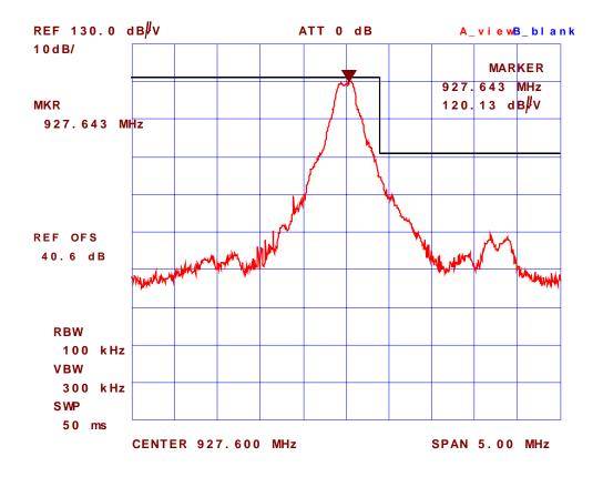
Plot #40:Band-Edge Radiated Emissions @ 3 meters, Rx Antenna: Vertical<br/>Test Configuration # 1: Microhard MHX920 with ¼ Wave Antenna, Microhard P/N:<br/>MHS031060, Gain: 1.5 dBi Microhard, Highest channel frequency: 927.6 MHz
