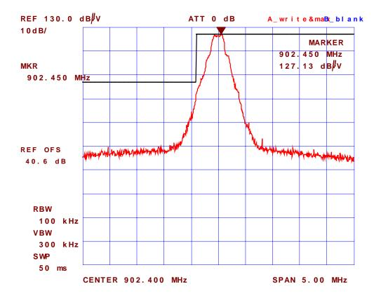
Plot #46: Band-Edge Radiated Emissions @ 3 meters, Rx Antenna: Vertical Test Configuration # 3: Microhard MHX920 with Transit Antenna, Microhard P/N: MHS031220, Gain: 3 dBd, Lowest channel frequency: 902.4 MHz
