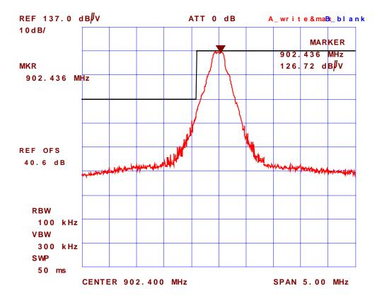
Plot #39: Band-Edge Radiated Emissions @ 3 meters, Rx Antenna: Horizontal Test Configuration # 1: Microhard MHX920 with ¼ Wave Antenna, Microhard P/N: MHS031060, Gain: 1.5 dBi Microhard, Highest channel frequency: 927.6 MHz
