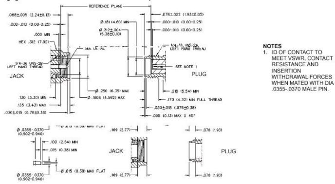
The RF connector on the module is an End Launch Reverse-Thread SMA Bulkhead Jack Receptacle. The manufacturer's part no. Johnson 142-5701-811.
