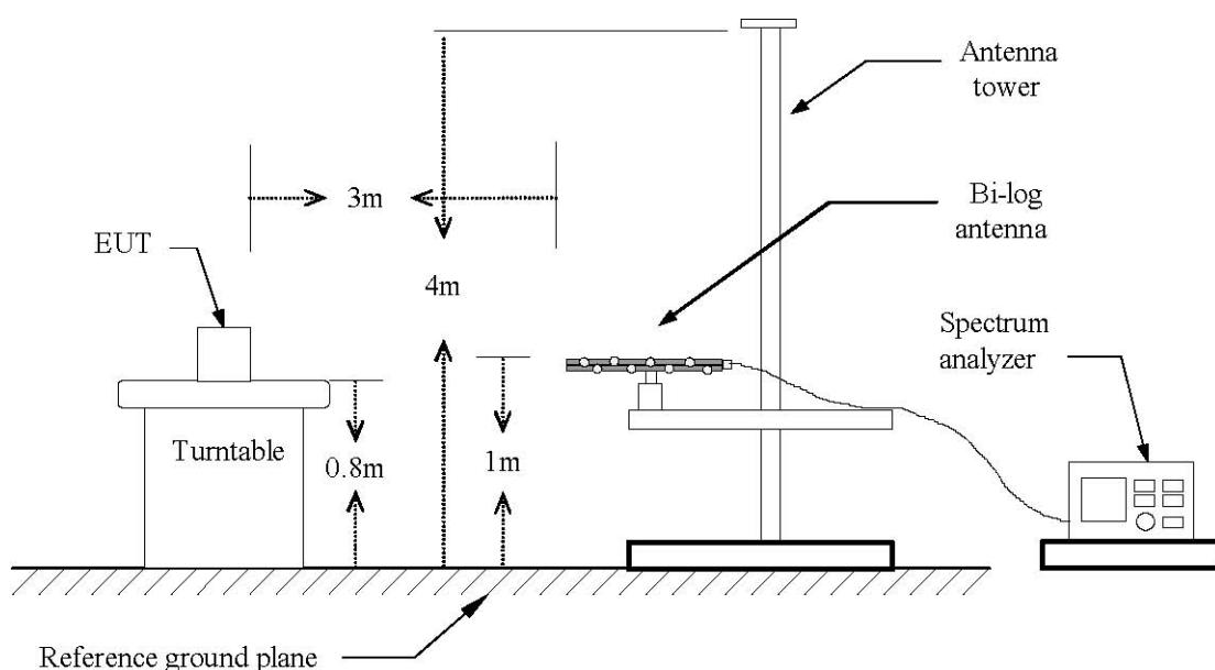
**Above 1 GHz**
