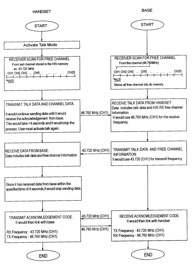
CONDITION 2 : Multi channel on the base TX frequency are occupied.
