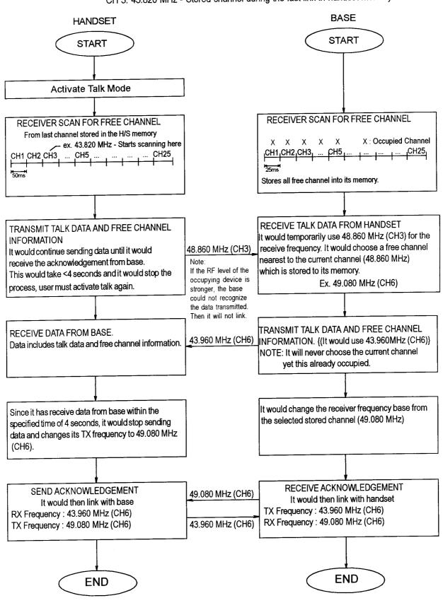
CONDITION 4 : Multi channel on the Base TX and Handset TX frequency are occupied.
