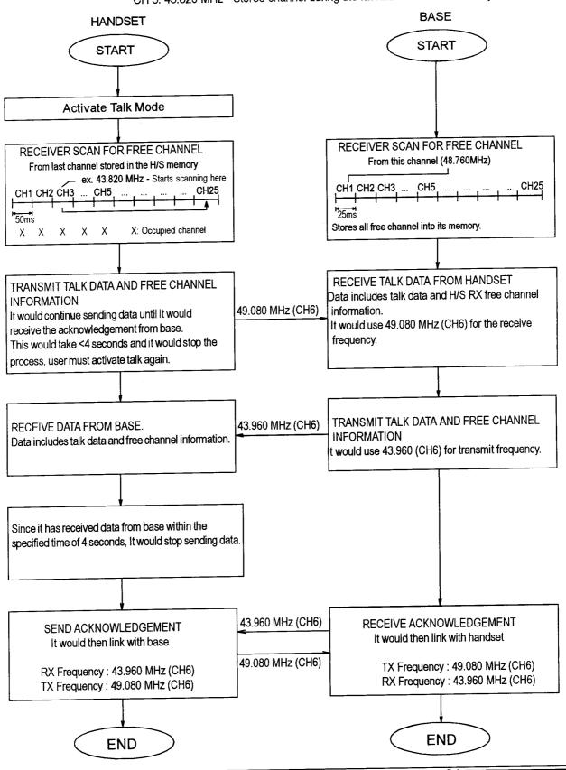
CONDITION 3 : Multi channel on the Handset TX frequency are occupied.
