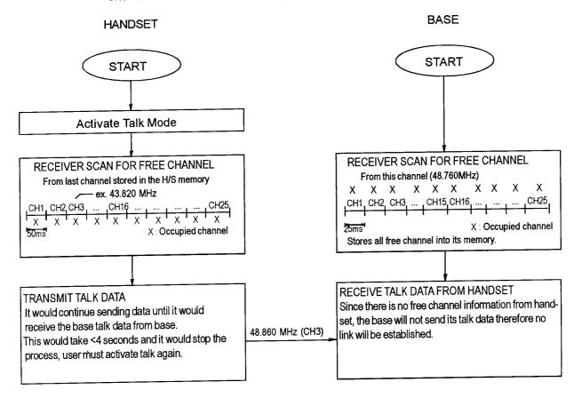
The above condition, if all transmit channels of Handset and Base are occupied (all busy), Handset will transmit the data using it's default channel. (NOTE: Default channel is the last link channel), Since the data does not contain free channel the base will not acknowledge, Therefore no link will be establish.
