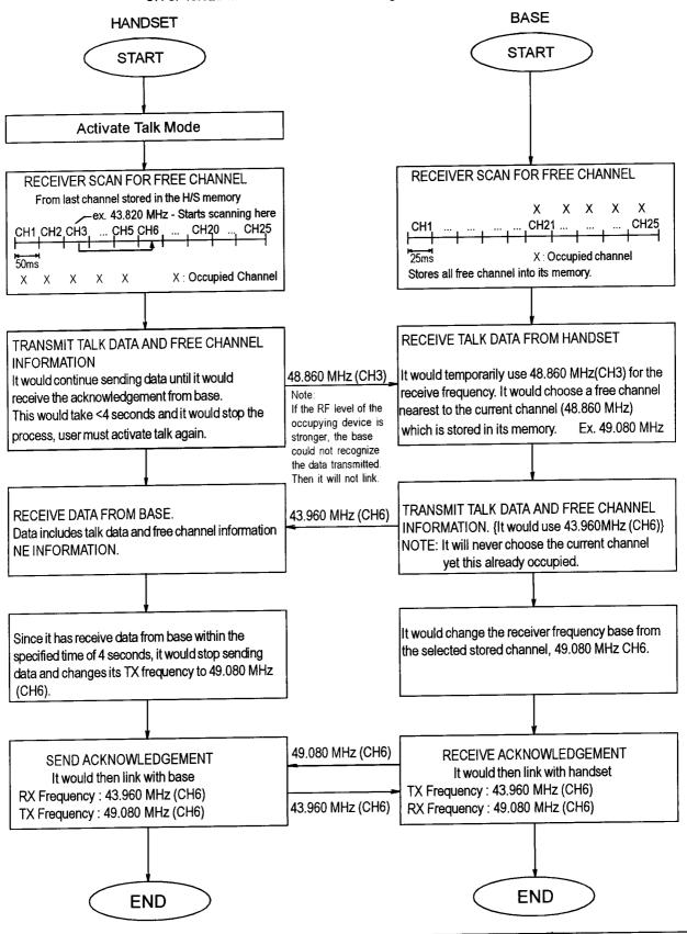
CONDITION 5 : All new TX channel (CH 1-15) of Handset and Base are occupied (All Busy)
