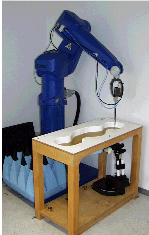
Fig. 2: The measurement setup with a phantom containing tissue simulating liquid and a device under test.
