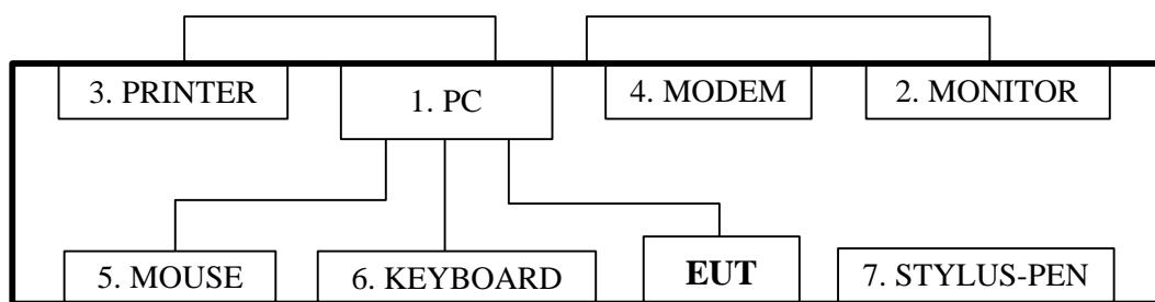
Both conducted and radiated testing were performed according to the procedures in ANSI C63.4:1992. Radiated testing was performed at an antenna to EUT distance of 10 m on an open area test site. Please refer to the photos of test configuration in Item 5.
