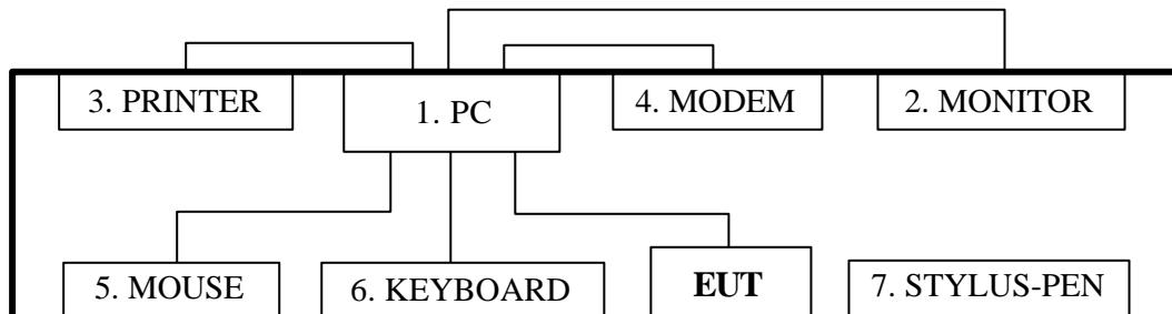
Both conducted and radiated testing were performed according to the procedures in ANSI C63.4:1992. Radiated testing was performed at an antenna to EUT distance of 10 m on an open area test site. Please refer to the photos of test configuration in Item 5.
